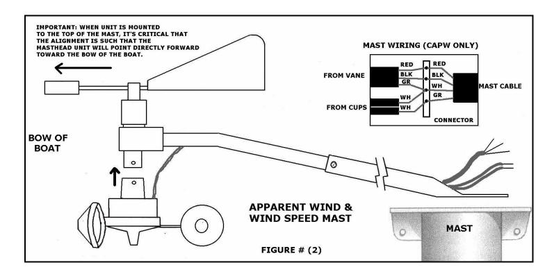
**DOUBLE CHECK ALL CONECTIONS!!!!** When satisfied that the wires are properly matched, connect the 4 pin connector halves together. It is recommended that the connector be waterproofed with a silicone compound where the cables enter the rubber boot. <u>Do not</u> use any silicone on the mounting pipes.
